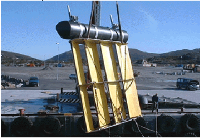
Figure 2 A concept for “door” on a seismic survey system. The “Barovan” (Baro 2008)
