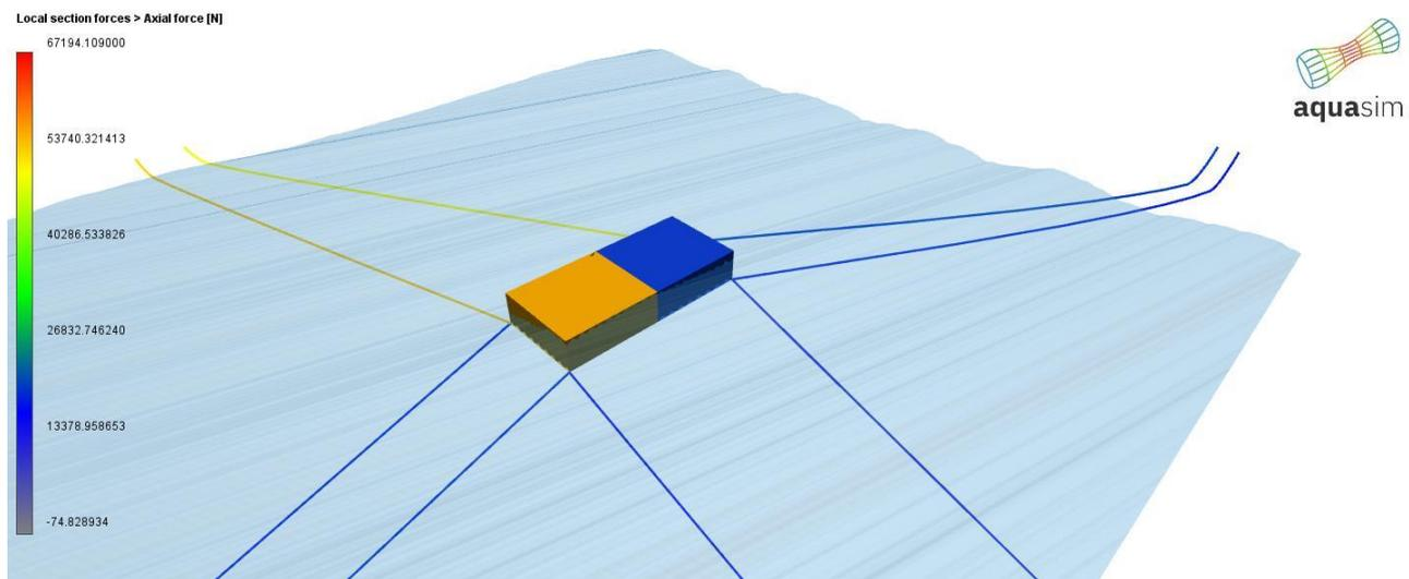
Figure 6 Axial forces in mooring lines
