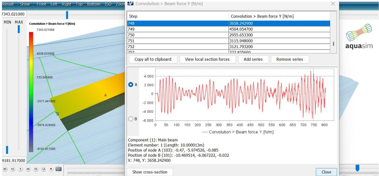
Figure 5 Convolution forces to beam.
