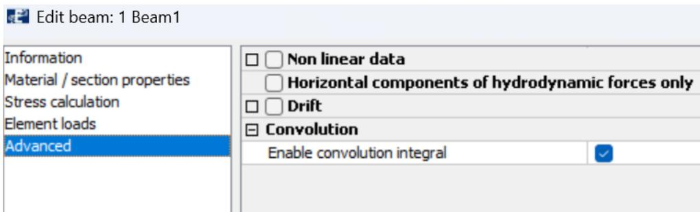
Figure 1 How to enable hydrodynamic damping by convolution
