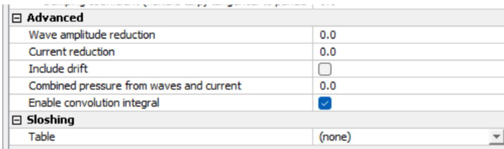
Figure 2 Enabling convolution for panels
