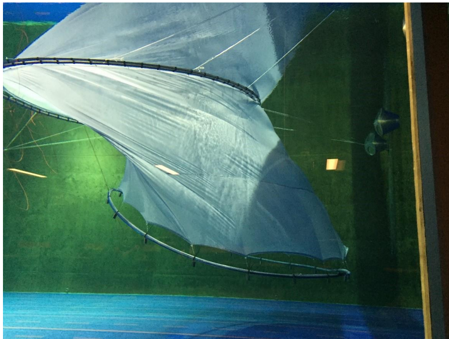
Figure 32 Tubenet exposed to 14.5 cm/s current
