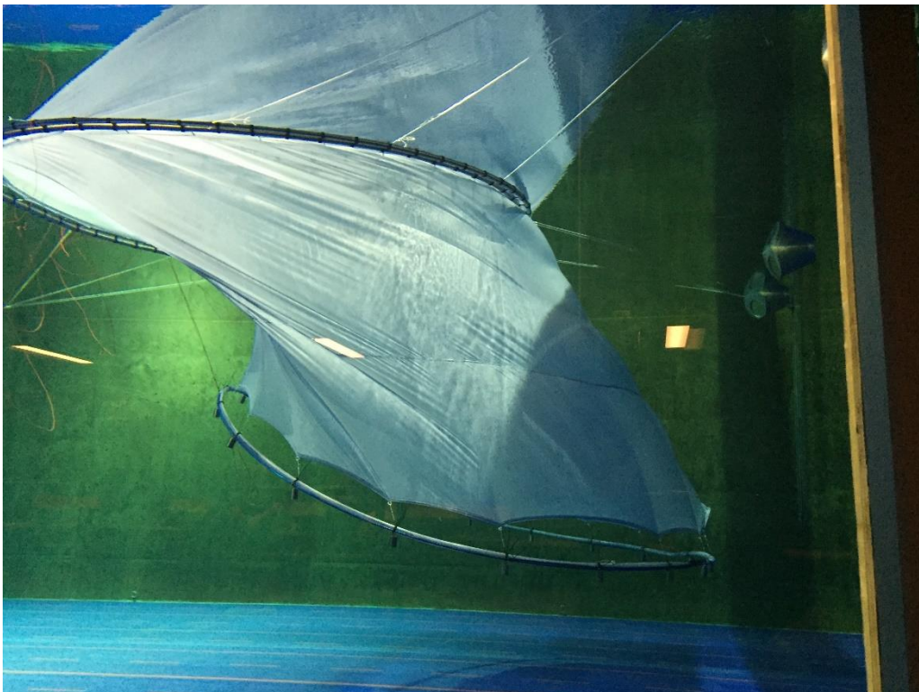
Figure 27 Tube exposed to 14.5 cm/s current
